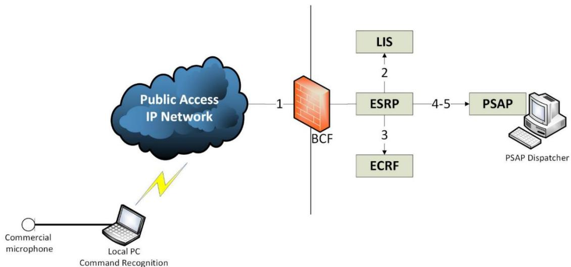
Figure 15: Command Recognition System (Integrated to NG112)
