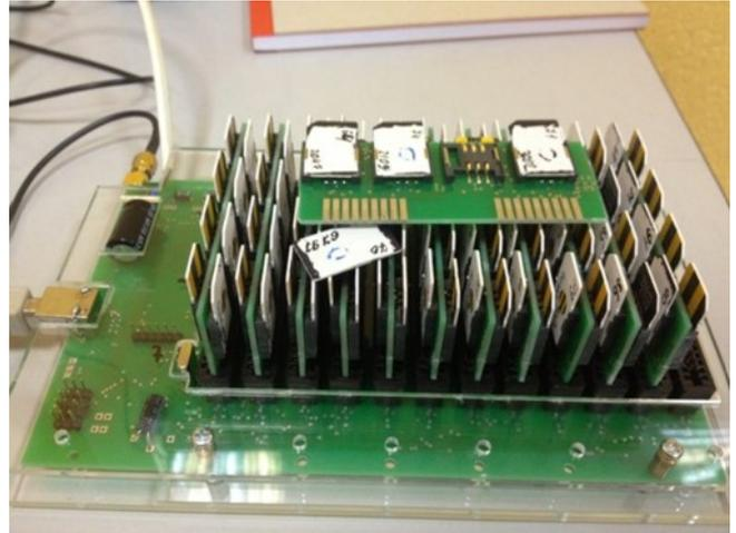
*Homemade device to generate TDoS attacks*
