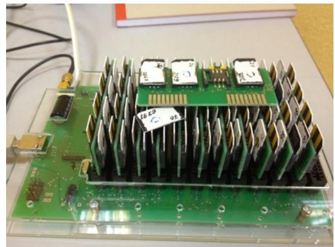
*Homemade device to generate TDoS attacks*
