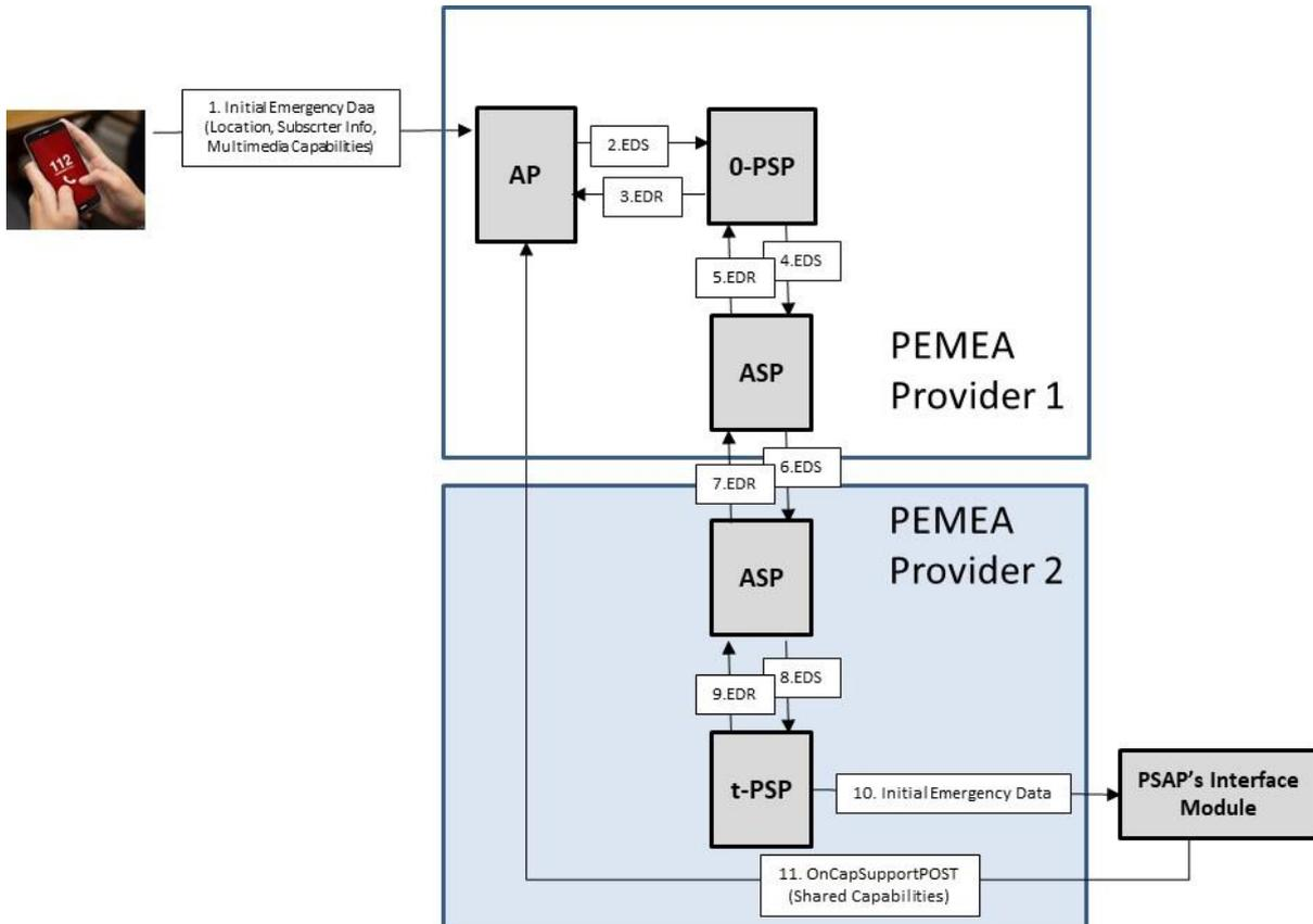
1. The App sends the initial emergency data to the AP including the user location and the multimedia capabilities it has, using the Pa interface.
