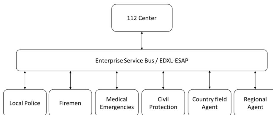
The objective was to make a flexible and configurable integration for new stakeholders. A media gateway is used for the integration of new emergency response organisations. Information about incidents are updated in real-time. This way, voice communication is not needed any longer.
