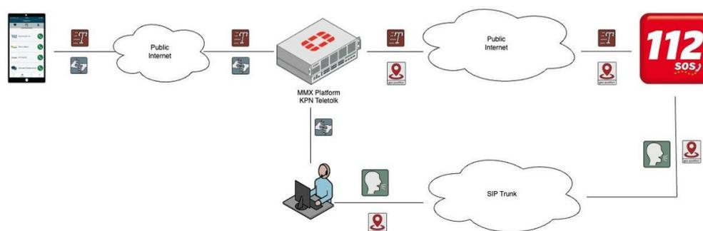
Figure 7: Call flow for text and video relay services in The Netherlands (source: nWise)
