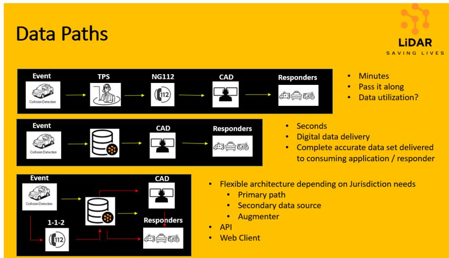
Figure 13: Data paths - Device to PSAP (source: LidarSavingLives)
