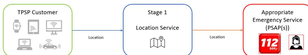
Figure 9: Delivering caller location to the right PSAP in real-time (source: SS8)
