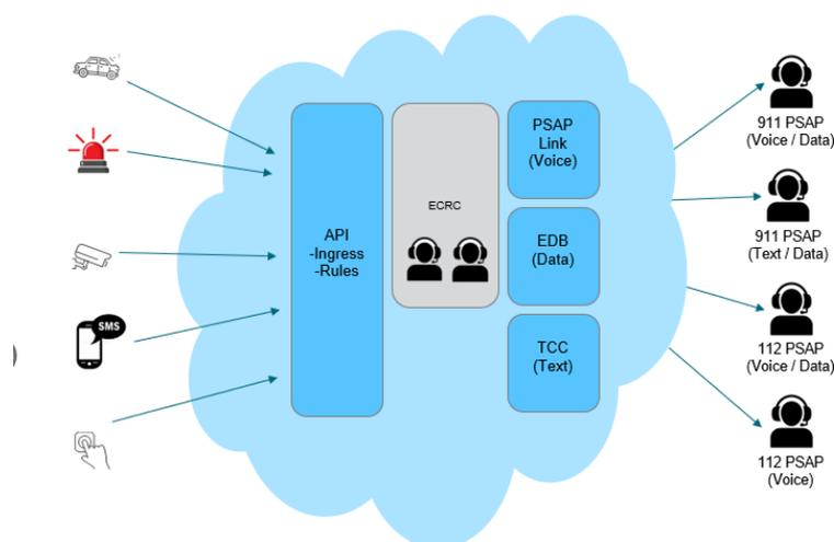
Figure 8: Channels used to contact PSAPs and provide contextual data using the Intrado Platform (source: Intrado)
