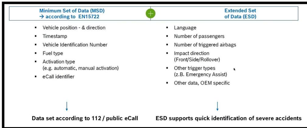
Figure 1: Contents of MSD and ESD for TPS eCall (source: Bosch Service Solutions)
