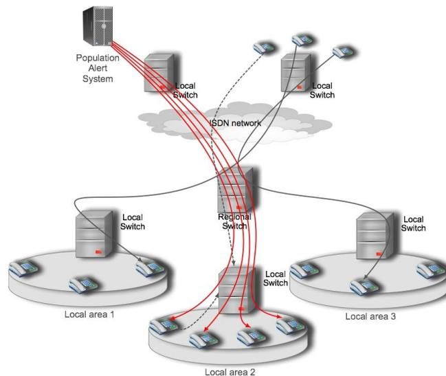
Figure 3: Structure of typical PSTN
