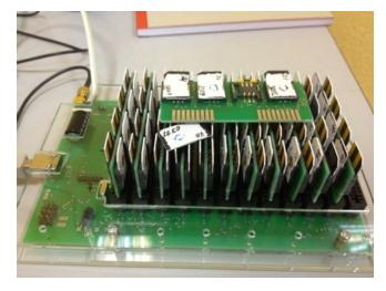
Homemade device to generate TDoS attacks
