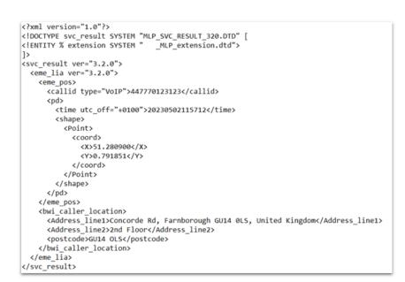
Figure 10: Geodetic location example (source: SS8)
