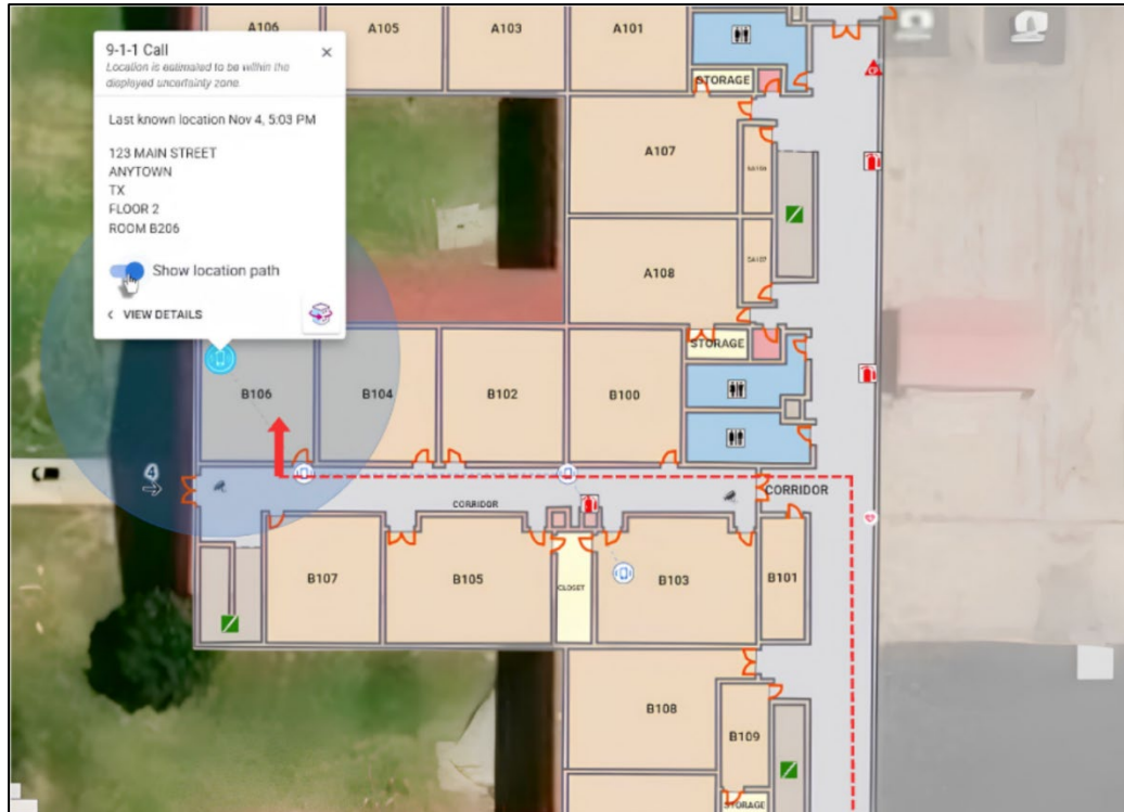
Figure 1. The location of an emergency call overlaid onto an indoor map. The blue dot represents the caller's estimated location, with the location's uncertainty represented by the transparent blue circle. The dashed red line indicates the optimal route that responders should follow to reach the caller's location. Image courtesy of GeoComm.
