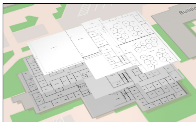
Figure 3. Three altitude-aware geo-referenced indoor maps, each representing a floor within a building, displayed in 3D. Image courtesy of Esri.
