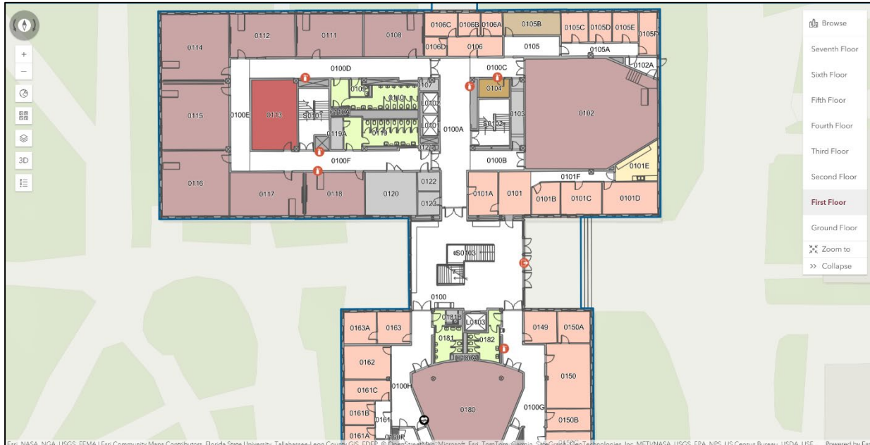
Figure 7. A floor-aware, vector GIS-based indoor map representing the first floor of a building. The map is shown in 2D, and maps of other floors can be displayed by selecting a floor on the upper right-hand side of the screen. Interior spaces are classified by use type and rooms are labeled with room numbers. The map also shows the location of fire hydrants, exits, and AEDs. Image courtesy of Map I.T.
