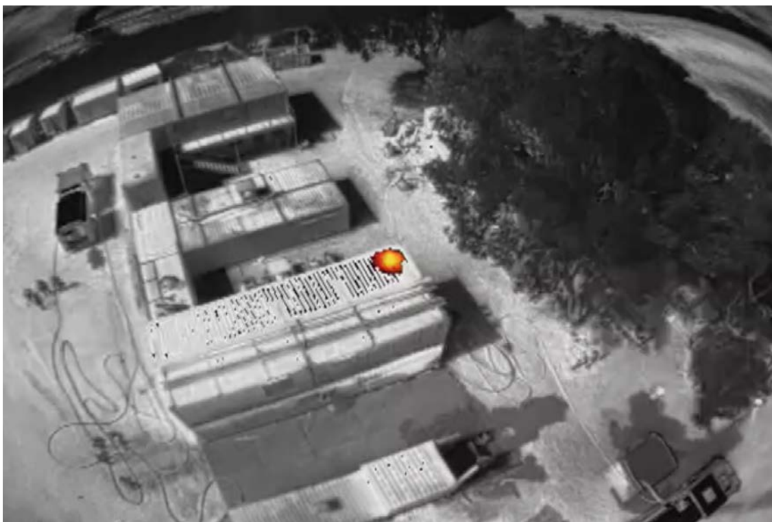
Example of structural fire as seen with the DJI XT thermal imaging camera and Isotherm settings ON.
