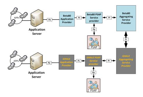
Figure 2 PEMEA-provider high-level interconnection
