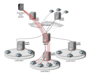
Figure 3: Structure of typical PSTN
